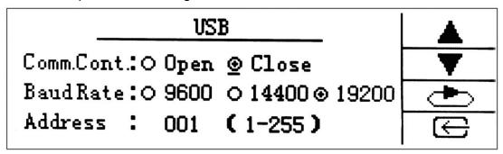
Equipment supported by the USB communication only refers to the using USB as a communication transmission medium, USB does not support U disk and other USB devices operation. Which contains the parameters as follows:
