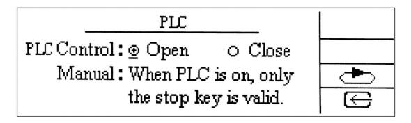
If the PLC interface is enabled, all the keys are invalid except reset button .then the instrument can be tested by the PLC.
