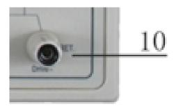
Secure the test line well at this point 10( return terminal)
