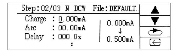
Charging current: Charging current upper limit alarm range: 0 to the current upper-limit alarm value, when the charge current upper-limit alarm value is set to 0, on behalf of the charging current upper limit alarm judgment is off.
