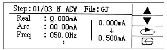
Real current: the real current upper limit alarm; real current upper-limit alarm range: 0 to current up-limit alarm value, when the real current upper limit alarm is set to 0, representative of the real current up-limit alarm is off.
