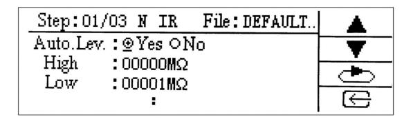
Automatic range: automatic range settings; This setting determines whether auto IR range in the testing process, if set on, auto range is on; if set No, then automatically shift IR range is off. Use IR low-limit value to determine range in testing process. Resistance up-Limit: When insulation resistance up-limit value is set to  $0M\Omega$ , on behalf of insulation resistance up-limit alarm is off.
