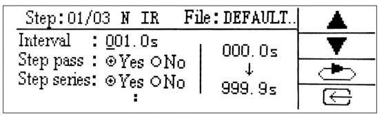
Interval time: interval time between the current test step; Range:  $0s \sim 999.9s$ , when the interval is set to 0s, a representative interval is off.
