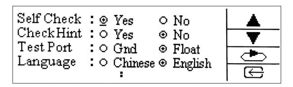
Verification allowed: set check; if the verification is turned on, then turn on the power, the tester will verify automatically.
