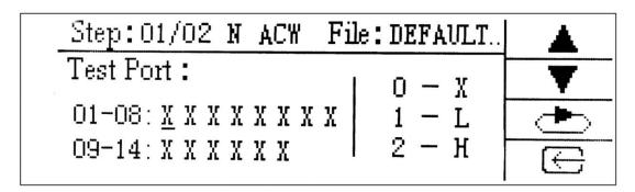
Test port: test port of the current test step; when the instrument model is CS9919AX,
