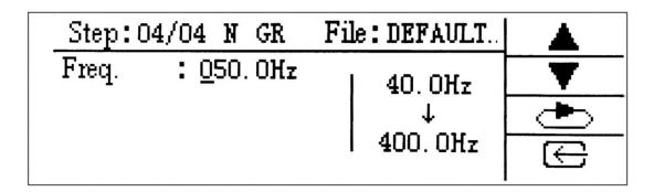
Output frequency: the current test step output frequency; range: 40.0Hz ~ 400.0Hz
