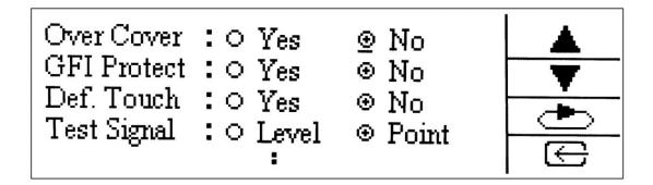
Over cover: overflow cover set; if overflow cover is turned on and the storage results are greater than 9999, the tester automatically save the results from the beginning; If the overflow cover is turned off, then discard the test results.
