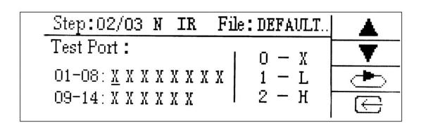
Test port: When the instrument model is CS9919AX, CS9929AX, CS9929CX, CS9919G, the tester has eight test ports. When the instrument model is CS9919BX, CS9929BX, the tester has four test ports. When the instrument model is CS9929EX, the tester has 14 test ports. Test port range: X - high impedance state, L – low level state, H - high level state.
